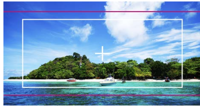
Aspect Mode: 2.35:1, Safe Area: Shape A, Area Size: 80%
