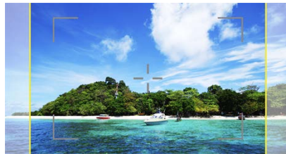
Aspect Mode: 14:9, Safe Area: Shape B, Area Size: 80%
